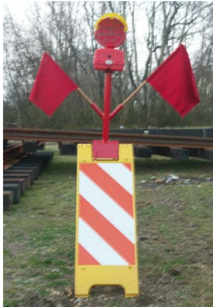
Simulating the end of train, this “banner” was used in a recent efficiency test.
