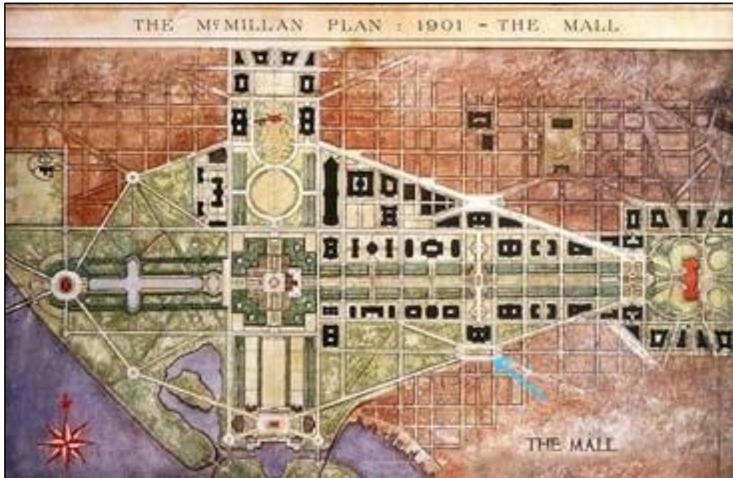
Figure 10. In the McMillan Plan's City Beautiful version of the Washington Mall, all trackage was removed, Maryland Avenue marked a break between park and city, Reservation 113 (blue arrow) reverted to public park, and the railroad corridor was out of sight. Source: Library of Congress.
