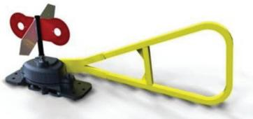
**Switch Target** – A switch target is a visual indicator to employees to tell the direction of movement the switch is lined for. When the switch stand is operated, the switch target automatically turns to correspond with the movement.
