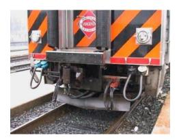
**Gauge –** The gauge of the track is the portion between the two rails. In North America, the width is 4' 8.5", which is considered the standard gauge.
